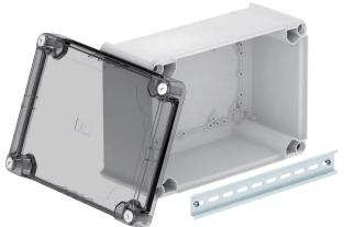
Closed junction box for the connection of cables and lines indoors and in protected outdoor areas. Rectangular design without entries. Suitable for wall and ceiling mounting, on mounting panels and threads in the floor. With the option to fasten inside and to mount via the corner domes. High, transparent cover with quick lock, sealable. Made from halogen-free materials. With hat profile rail.
