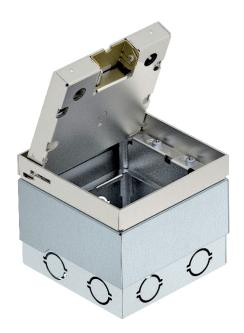
Square floor socket with floor covering recess for use in dry-care cavity and screed floors for indoor use. Installation housing with pre-marked insertion openings for pipelines (M25). Cover adjustable to the top edge of the floor covering using four height-adjustment supports. The minimum installation depth is 110 mm, the height-adjustment range + 20 mm. Surfaces visible in the floor covering made of: Stainless steel.
