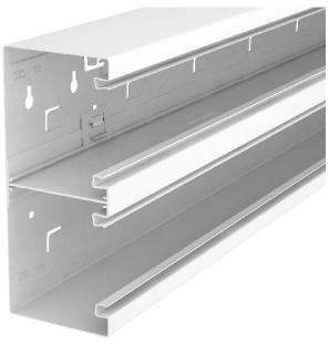
GS device installation trunking for mounting on the wall or on fastening panels. The GS device installation trunking possesses self-contacting locking straps to accept a sheet steel partition. The equipotential bonding between the trunking bases takes place using the trunking coupler. The protective measure and the equipotential bonding is guaranteed between the cover and the base by the self-contacting trunking cover. The real system opening is 76.5 mm.
