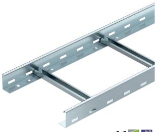
Cable ladder with perforated side rail of side height 60 mm with riveted C profile frames, open in an upwards direction (VS version).
