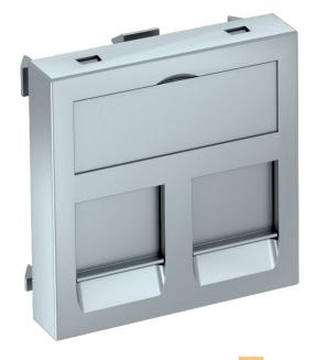
Data technology support with straight outlet and locking slider to accept two data technology connection modules with RJ45 socket. The locking fastening is suitable for horizontal and vertical installation in the system environment. Type PA has a special module seat and is designed for indirect fastening of the data connection modules in the mounting opening.
