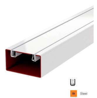
Four-sided, metal fire protection duct to install and route cables. With intumescent inner lining. In the event of fire, it prevents the spread of fire in the duct and protects emergency and escape routes against the impacts of a cable fire.
