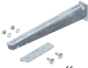
Bracket for mounting on suspended supports or as wall bracket for cable tray routing type above fire protection ceilings and for routing types with cable ladders and cable trays for the maintenance of electrical function according to DIN 4102 Part 12. The brackets are supplied ready-mounted.
