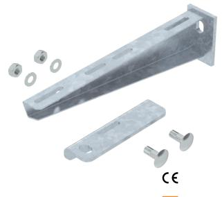
Bracket for mounting on suspended supports or as wall bracket for cable tray routing type above fire protection ceilings and for routing types with cable ladders and cable trays for the maintenance of electrical function according to DIN 4102 Part 12. The brackets are supplied ready-mounted.
