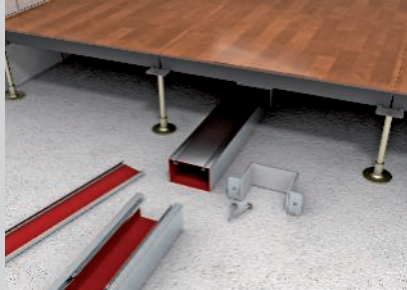
Mounting on raw concrete in system base.
