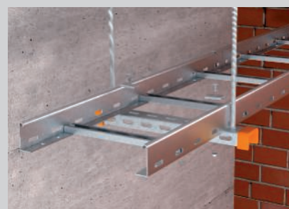
Mounting on transverse profile with clamping piece, truss-head bolts and large washers.
