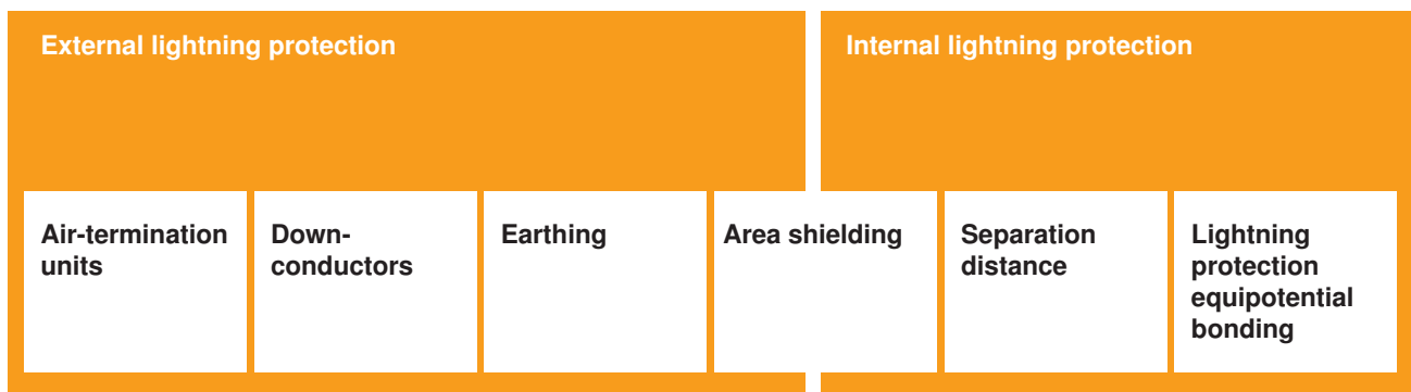
External and internal lightning protection systems
