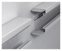
**GK coupling mounting** The coupling of the GK device installation trunking is contained in the scope of delivery and is pre-mounted. It is pulled out of the trunking and automatically locks in the correct position. This allows simple mounting of additional trunking sections.
