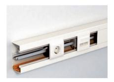
The installation of an accessory mounting box reduces the usable cross-section available for cable routing. The value "net" in the tables indicates this usable trunking cross-section.
