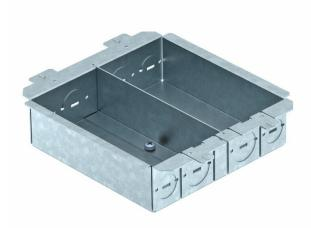
Closed mounting support to accept 2 APMT2 cover plates. The mounting support is fastened below the GES4DB service outlet. Each with 4 knock-out openings M20 and M25 for the mounting of flexible installation hoses.
