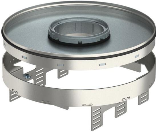
Height-adjustable cassette, decoupled from the floor, of nominal size R9, for tube bodies, for the installation of accessories in dry or wet-cleaned floors for indoor use, for mounting in underfloor boxes UZD350-3, either in conjunction with a mounting lid DUG350-3R9 or UGD350-3R9. Mounting takes place using height adjustment brackets (order separately) in the aluminium frame profile of the underfloor boxes.
