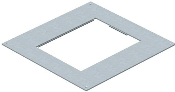
Mounting lid for underfloor junction and branch box of type UZD250-3/4 for the installation of an installation unit of nominal size 6. Installation opening 3 mm recessed for later blanking lock with lid blind plate.
