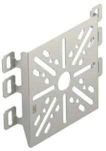
Mounting plate, for fastening on the side rail of cable support systems. Fastening on the side rail of the mesh cable tray is carried out without bolts by bending the lugs. Fastening on the side rail of cable trays or cable ladders is carried out with two truss-head bolts. Type B9/T junction boxes can be mounted very easily by inserting the bolt plug supplied into the centre hole on the mounting
