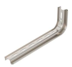
TP support / bracket for the fastening to horizontal concrete ceilings and walls. If the profile is fastened directly to the ceiling or the profile is screwed together as head reinforcement, then, for reasons of stability, always use the spacer, type DS
