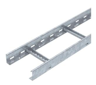
Cable ladder with a 60 mm side height with welded C30 profile rungs which are open in an upwards direction. Rolled side rail for reinforcement and as edge protection. Fastening to the bracket takes place using hold-down clamps, type LKS 40. The slot dimension of the rung is 16.5 mm and the appropriate clamp clip is type BS-H....
