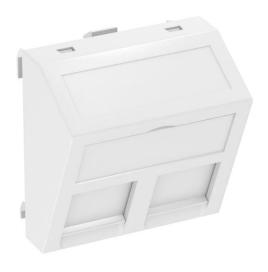
Data technology support with slanting outlet and locking slider to accept two data technology connection modules with RJ45 socket. The locking fastening is suitable for horizontal and vertical installation in the system environment. Type A has a mounting opening of 20.10 x 14.80 mm and is designed for direct fastening of the data connection modules in the mounting opening.
