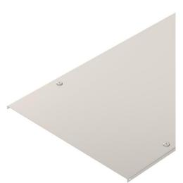
Cover for cable trays and cable ladders with three pairs of turn-buckles. When using covers outdoors, additional measures against the influence of wind must be taken. Cover clamps or turn buckles on their own are not sufficient securing elements against wind loads.
