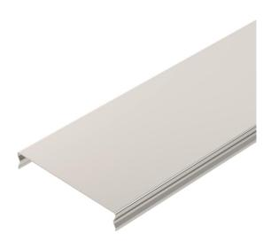
Snap-on cover for mesh cable trays. Protects cables from damage, contamination and moisture from above. Suitable for the foodstuffs or chemicals industries. With transverse bead from 16 in. width.
