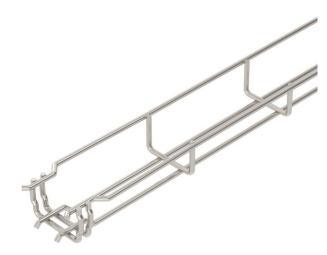
Patented, snap-together wire mesh cable tray system enables the contractor to connect and install tray 50% faster than traditional wire mesh. GR-Magic eliminates the need for additional connection hardware when connecting full length sections together. Tray side-height is 1 in.
