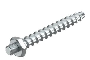
Bolt tie for direct mounting without additional anchors in cracked and uncracked concrete and masonry. M6 connection thread for fastening clips with threaded foot
