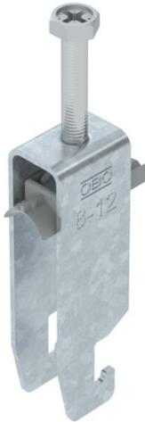
Clamp clip with U-foot, plastic pressure sleeve made of polypropylene. For vertical and horizontal mounting of 3 single cables on a C-profile rail. For slot width 18 mm or 22 mm. With 1-start screw thread on pressure sleeve, universal hexagonal screw head WAF10, with slot and cross recess. Suitable for assembly indoors and outdoors. Multiple cables should be separated by double sleeves. We recommend the use of a counter-sleeve.
