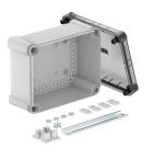
Junction box with hat profile rail for the connection of cables and lines indoors and in outdoor areas. Rectangular design without entries. Suitable for wall and ceiling mounting with the option to fasten outside, inside or to mount via the corner domes. Particularly impact resistant with IK09. Transparent cover with quick lock, sealable. Made from halogen-free and UV-resistant materials.
