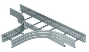
Horizontal T branch piece, for all wide span cable ladders of 160 mm side height. For further stabilisation, additional supports should be planned for the area of the fittings.
