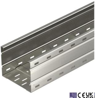
Wide span cable tray system, perforated, with a side height of 160 mm. Straight connectors of type WRVL 160 should be ordered separately and in the appropriate quantity. Magnetic shield insulation without cover 20 dB, with cover 50 dB.
