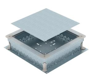
Underfloor junction and branch box for 10 installation pipes on each side (M20 or M32) with sheet steel side walls. To mount installation units in the mounting lid (to be ordered separately). Height can be infinitely adjusted to the nominal screed height (rapid adjustment possible) and the screed can be worked flushed to the screed scraping edge. With noise decoupling option after screed laying and can be used with system accessories, also for heavy-duty application.
