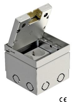
Square floor socket with floor covering recess for use in dry-care cavity and screed floors in indoor areas. Installation housing with pre-marked insertion openings for pipes (M25). Cover adjustable to top edge of floor covering using four height-adjustment supports. The minimum installation depth is 110 mm, the height-adjustment range + 20 mm.
