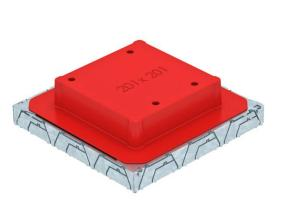
Underfloor outlet box with fixed, unchangeable 201 x 201 mm installation opening for an installation unit of nominal size 4. The mounting opening is created using the screed protection cover contained in the scope of supply. The underfloor box possesses installation openings for three single-compartment PVC ducts of nominal size 60 x 25 and 90 x 35 on all four sides. The box is principally suited for use in floor structures in cement screed with a structure height of up to 90 mm.
