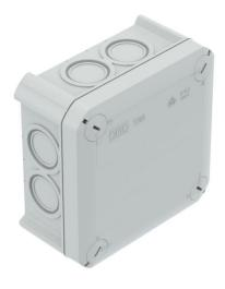
Junction box for the connection of cables and lines indoors and in protected outdoor areas. Square design with knock-out entries to the sides and knock-out entries in the bottom. Suitable for wall and ceiling mounting and on mounting panels. With the option to fasten inside and to mount via the corner domes. With fixed clamping cover. Made from halogen-free and UV-resistant materials.
