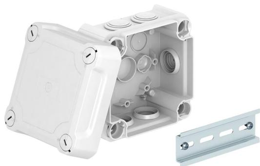
Junction box for the connection of cables and lines indoors and in protected outdoor areas. Square design with plug-in seals to the sides and knock-out entries in the bottom. Suitable for wall and ceiling mounting and on mounting panels. With the option to fasten inside and to mount via the corner domes. High cover with quick lock, sealable. Made from halogen-free and UV-resistant materials.
