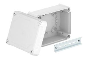
Closed junction box for the connection of cables and lines indoors and in protected outdoor areas. Rectangular design without entries. Suitable for wall and ceiling mounting and on mounting panels. With the option to fasten inside and to mount via the corner domes. High, transparent cover with quick lock, sealable. Made from halogen-free and UV-resistant materials.
