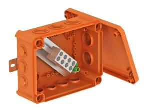
Halogen-free junction box with pre-mounted, soft plug-in seals, approved for the maintenance of electrical functionality according to DIN 4102 Part 12. Maintenance of electrical functionality classes E30 to E90.
