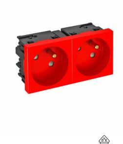
Socket with earthing pin and side connection, Double 33°, with increased touch protection, with screwless terminals, 2-pin, 16 A, 250 V~, with connection terminals to IEC 60884-1.
