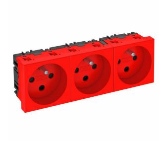
Socket with earthing pin, triple 0°, encoded version, with increased touch protection, with screwless terminals, 2-pin, 16 A, 250 V $\sim$ , with connection terminals according to IEC 60884-1.
