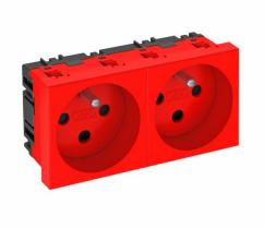
Socket with earthing pin, double  $0^\circ$ , encoded version, with increased touch protection, with screwless terminals, 2-pin, 16 A, 250 V~, with connection terminals according to IEC 60884-1.
