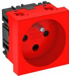
Socket with earthing pin, single 0°, encoded version, with increased touch protection, with screwless terminals, 2-pin, 16 A, 250 V~, with connection terminals according to IEC 60884-1.
