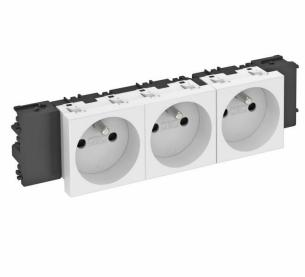
Earthing pin socket with connection to side, Triple  $0^\circ$ , with increased touch protection, with screwless terminals, 2-pin, 16 A, 250 V~, with connection terminals to IEC 60884-1, suitable for the installation in Rapid 45 device installation trunking systems.
