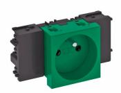
Earthing pin socket with connection to side, Single  $0^\circ$ , with increased touch protection, with screwless terminals, 2-pin, 16 A, 250 V~, with connection terminals to IEC 60884-1, suitable for the installation in Rapid 45 device installation trunking systems.
