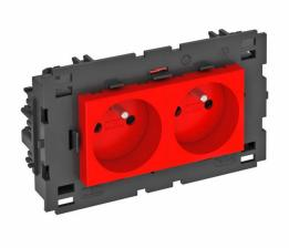
Socket with earthing pin with side connection Double  $0^\circ$ , with increased touch protection with screwless terminals, 2-pin, 16 A, 250 V $^\circ$ , with connection terminals to IEC 60884-1, suitable for installation in Rapid 80 device installation trunking systems.
