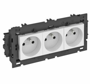
Earthing pin socket with connection to side, Triple 0°, with increased touch protection, with screwless terminals, 2-pin, 16 A, 250 V~, with connection terminals to IEC 60884-1, suitable for the installation in Rapid 80 device installation trunking systems.
