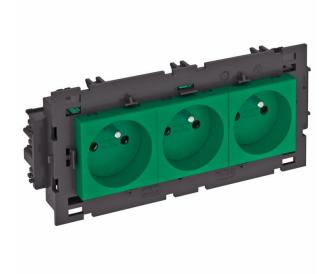
Earthing pin socket with connection to side, Triple  $0^{\circ}$ , with increased touch protection, with screwless terminals, 2-pin, 16 A, 250 V~, with connection terminals to IEC 60884-1, suitable for the installation in Rapid 80 device installation trunking systems.
