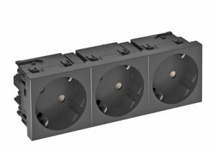
Power socket with side connection Triple 33°, with increased touch protection with screwless terminals, 2-pin, 16 A, 250 V~, with connection terminals to IEC 60884-1.
