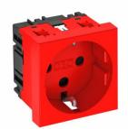
Protective contact socket, single 0°, encoded version, with increased touch protection, with screwless terminals, 2-pin, 16 A, 250 V $\sim$ , with connection terminals according to IEC 60884-1.
