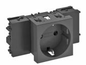
Protective contact socket with connection to side, Single 0°, with increased touch protection, with screwless terminals, 2-pin, 16 A, 250 V~, with connection terminals to IEC 60884-1, suitable for the installation in Rapid 45 device installation trunking system.
