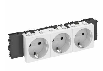
Protective contact socket with connection to side, triple  $0^{\circ}$ , with increased touch protection, with screwless terminals, 2-pin, 16 A, 250 V~, with connection terminals to IEC 60884-1, suitable for the installation in Rapid 45 device installation trunking systems.
