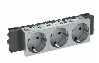
Protective contact socket with connection to side, triple  $0^{\circ}$ , with increased touch protection, with screwless terminals, 2-pin, 16 A, 250 V~, with connection terminals to IEC 60884-1, suitable for the installation in Rapid 45 device installation trunking systems.
