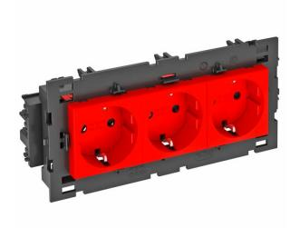
Protective contact socket with connection to side, triple  $0^{\circ}$ , with increased touch protection, with screwless terminals, 2-pin, 16 A, 250 V~, with connection terminals to IEC 60884-1, suitable for the installation in Rapid 80 device installation trunking systems.
