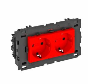
Protective contact socket with connection to side, double 0°, with increased touch protection, with screwless terminals, 2-pin, 16 A, 250 V~, with connection terminals to IEC 60884-1, suitable for the installation in Rapid 80 device installation trunking systems.
