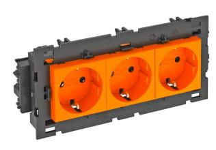
Protective contact socket with connection to side, triple 0°, with increased touch protection, with screwless terminals, 2-pin, 16 A, 250 V~, with connection terminals to IEC 60884-1, suitable for the installation in Rapid 80 device installation trunking systems.
